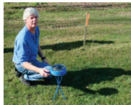
Local 673 member and JATC Instructor Ken Farabaugh demonstrates to his Solar Photovoltaic class how to set up the Sun Path Calculator, used to evaluate shading at potential array locations.
